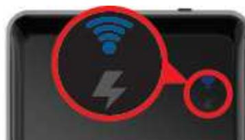
Flashing red indicates 25% battery charge remaining, turning to solid red when level reaches 20%. When using the App, a pop-up message will also indicate Low Battery status.
